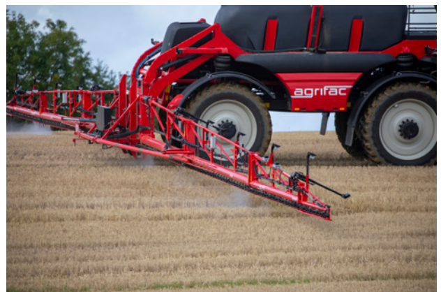
These are sent to the sprayer, which, thanks to the DynamicDosePlus system, sprays pointlike only in places where undesirable plants have been detected.
