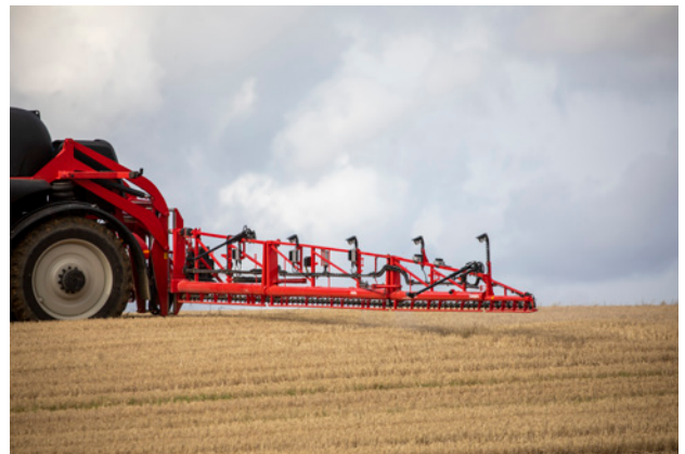
Condor Endurance II is equipped with the AiCPlus system built of cameras mounted on the spraying boom, which processes and analyzes the collected information in real time.
